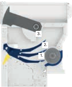
Hydraulic door for maintenance and removal of non-shreddables
