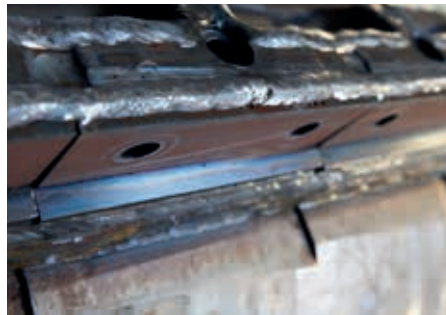
Rotor with blade knives – four-fold usable
