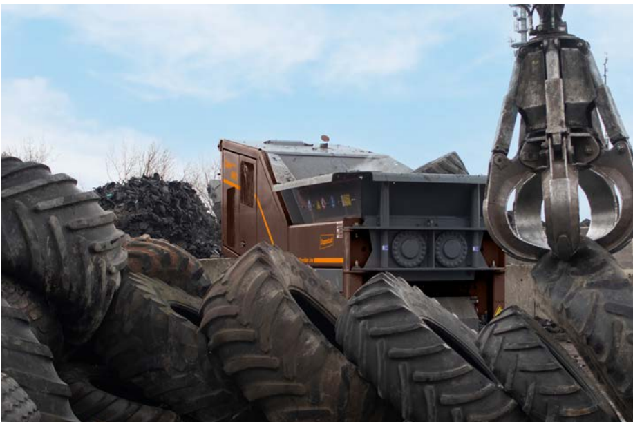
2 CoreShred 800 The mobile twin-shaft shredder in the medium performance class.
