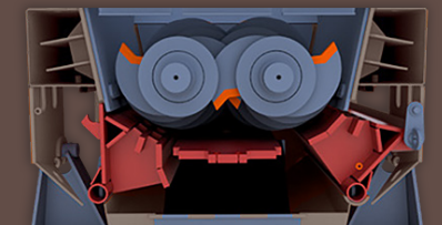
MECHANICALLY ADJUSTABLE COUNTER COMBS CoreShred 250 and CoreShred 800
