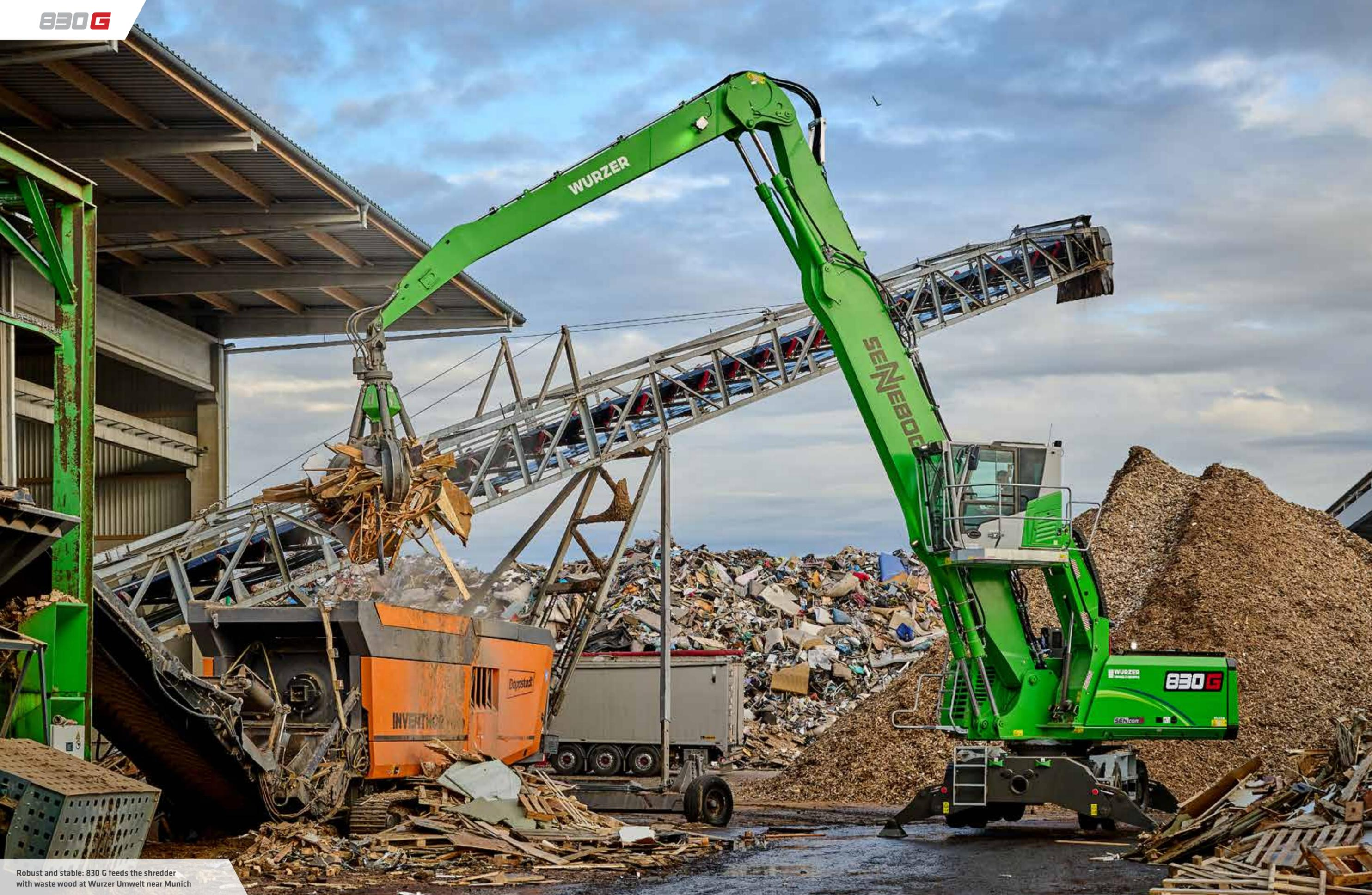
Robust and stable: 830 G feeds the shredder with waste wood at Wurzer Umwelt near Munich
