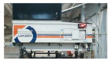
The new machine will allow meticulous and functional mixing of organic waste, green waste, soil, bark mulch and sludge to obtain the required matrix. This mixer can be used in different types of plants such as mechanical biological treatment, anaerobic digestion and composting.
