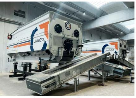
The UM 320 was developed out of this necessity, based on the experience of the last 20 years and is characterized by a robust steel construction, the special shape and dimensions of the mixing shafts and a powerful and reliable drive system. The accessibility of the mixing chamber from both sides, thanks to the opening through two large doors, allows a quick, safe and user-friendly service.
