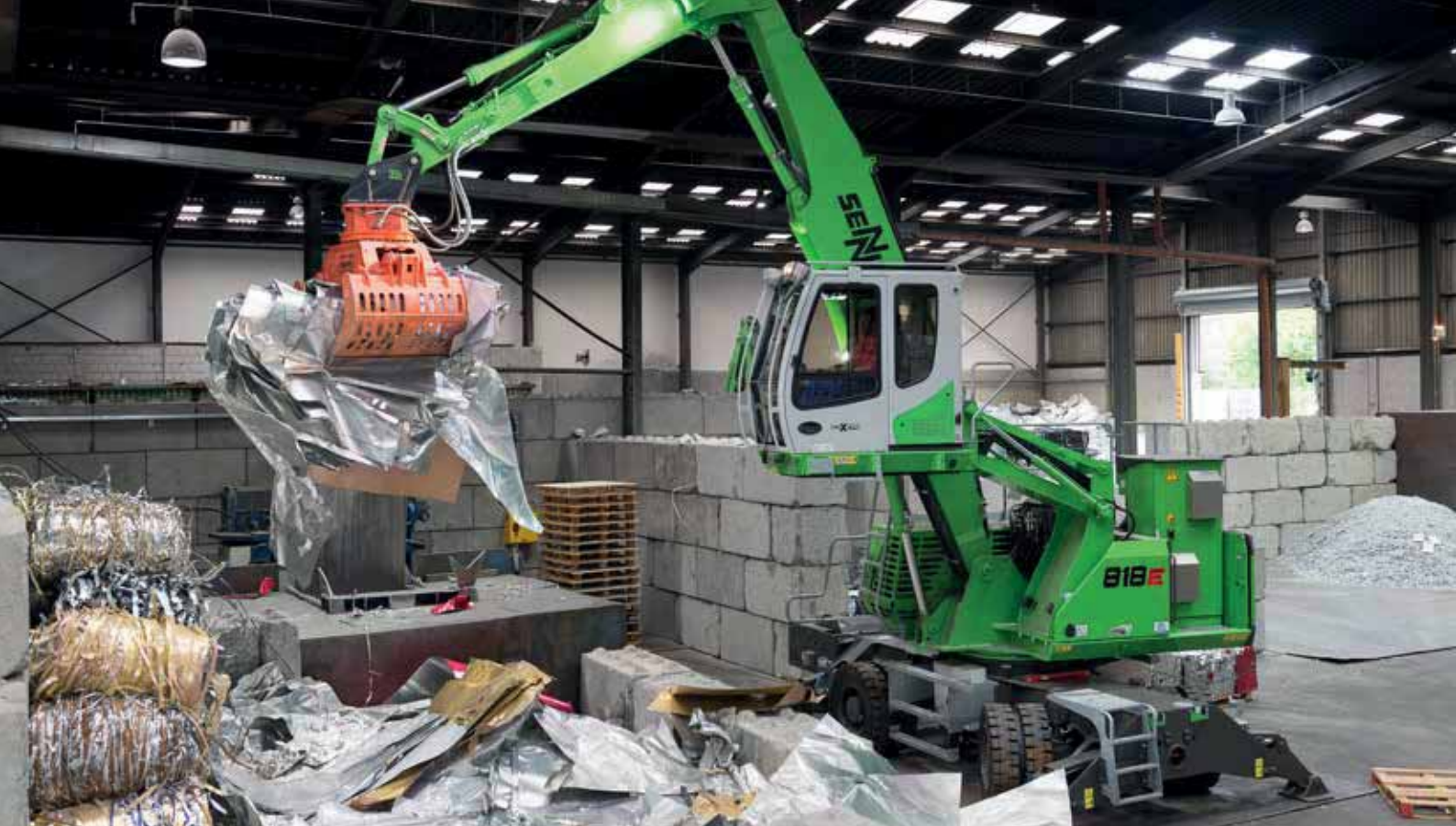
818 M Electro - Loading of a baler with sorting grab
