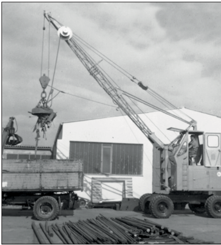
1962: rope-driven S833 with elevated operator cab
