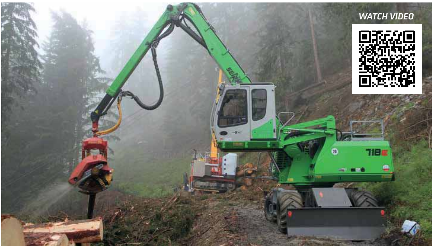
Cable yarding operation with harvester unit
